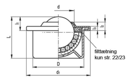
$$\begin{array}{ll} d & = 15.8 \\ D & = 24 \\ d1 & = 31 \\ L + -0.3 & = 21.0 \\ l1 + -0.3 & = 9.5 \\ l2 + -0.3 & = 5 \\ l3 & = 2.5 \\ Max load (N) = 500 \end{array}$$
